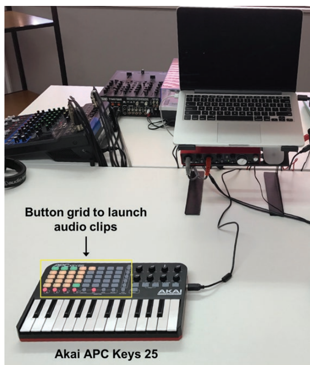
Figure 3. Desk set up for Clip-Jamming procedure showing Akai APC Keys 25 and trigger pads.
